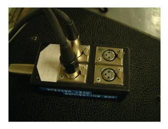
Note that the picture shows two speakers connected in positions 1 & 2. The other two speakers should be plugged in 3 & 4. Do not use 1 on it's own or 1&3 or 2&4 as these combinations won't work.
