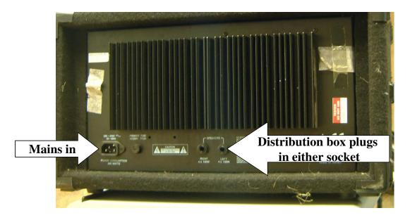
4. Each speaker cable is plugged into the speaker distribution box.
